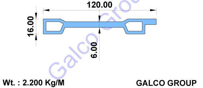
**BUILDING & CONSTRUCTION****SCAF FOLDING & FORMWORK****DIE NO. : 95728**
